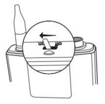
To turn on this Lavalier microphone flip the switch at the top to the **ON** position.
