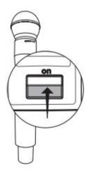
To turn on this Hand Held microphone flip the switch to the **ON** position.
