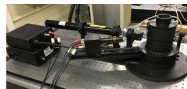
Backscattering DLS instrument for analysis of nontransparent samples
